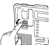
Tuck the telephone line cord inside the wall mounting adaptor, and push it in the direction of the arrow.
