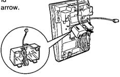
3 Connect the telephone line cord. Mount the unit, and slide down.
